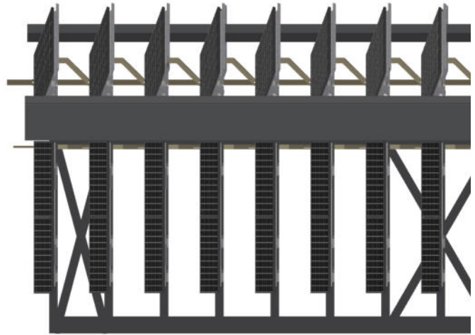
Figure: STE side view with opened PV modules
