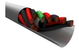
The division of the power cables into several small individual ones and the stranding of these individual wires results in a high flexibility of the charging cable. In the center of the cable is the supply line for the coolant, which flows back between the individual, insulated cores. This provides excellent cooling and high flexibility of the cable. In combination with the paXos charging plug, a particularly powerful and convenient charging system is provided.
